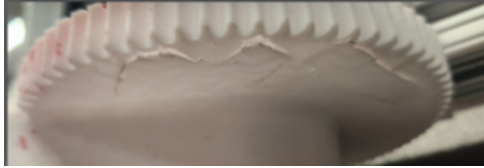
Figure 6: Cracking on Surface of Arm Stage 1 Gear
