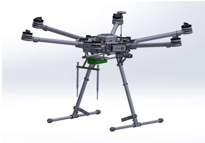
Figure 7. 3D Model of the SDR mounted on the antenna holder on the drone.
