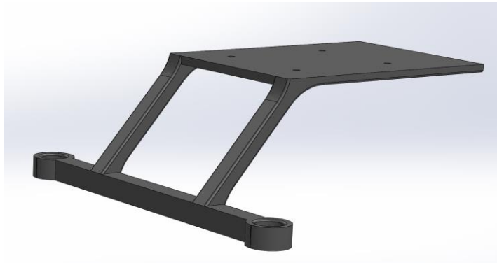
Figure 6. 3D Model of phased array antenna holder.
