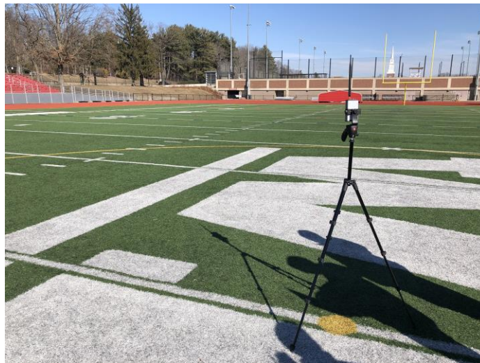
Figure 30. Transmitter setup for the football field test.
