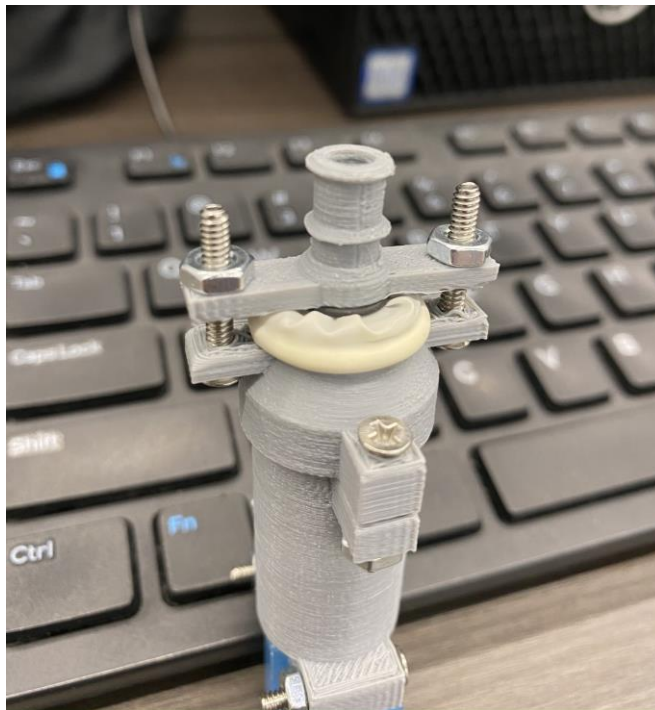
Figure 19: Prototype of O-ring nozzle concept used for testing
