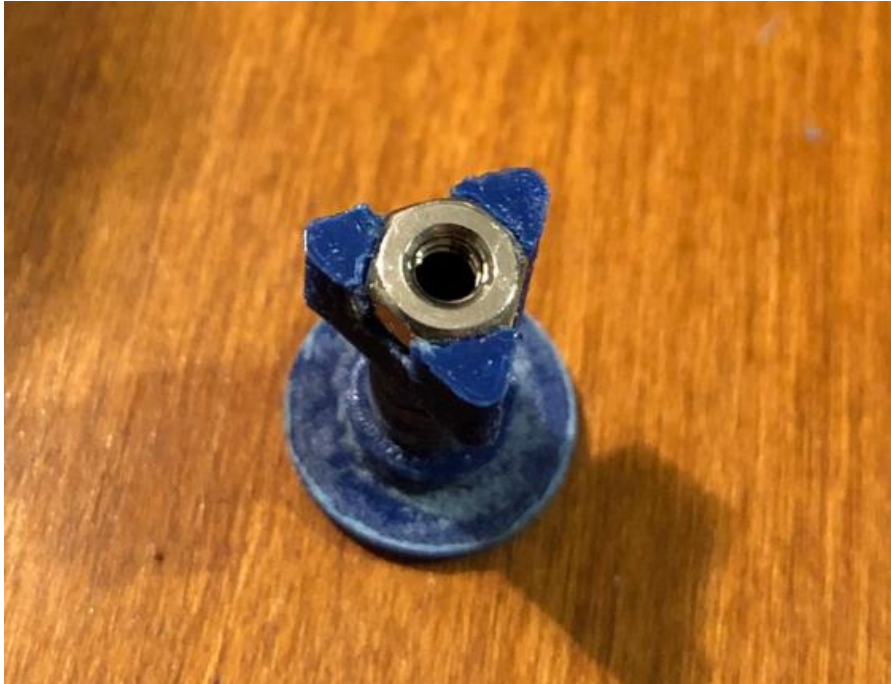
Figure 16: Nut glued into bottom of actuator plunger. Note the sanded edge of the circular portion
