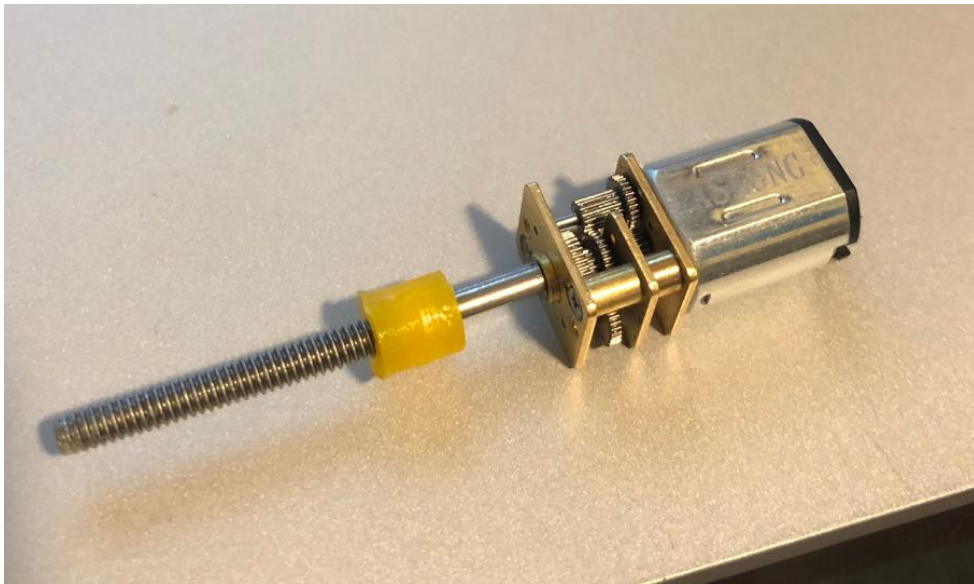
Figure 15: 3-D printed motor coupler
