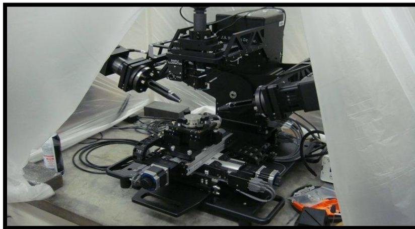
**Figure 8: M-2000<sup>®</sup> Ellipsometer**
