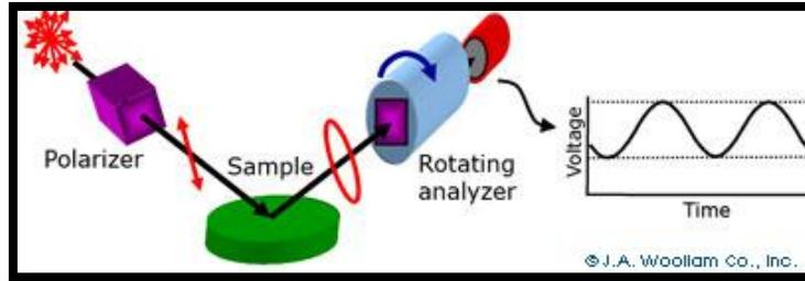
**Figure 7: Experimental Set-up for RAE Configuration (J.A. Woollam, 2010)**
