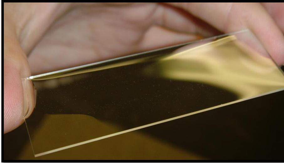
**Figure 14: Sample after dipping method was done. From the image, one will notice that the slide does not have much solution on its surface and that more collected on the right end versus being even over the surface.**
