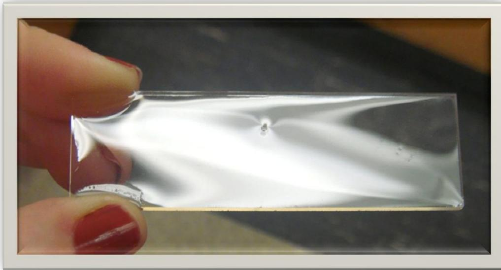
**Figure 15: Sample prepared using the pipette method. As stated, one of this method's flaws is that it can cause air bubbles on the surface of the slide, which could cause fluctuations in the ellipsometry data.**
