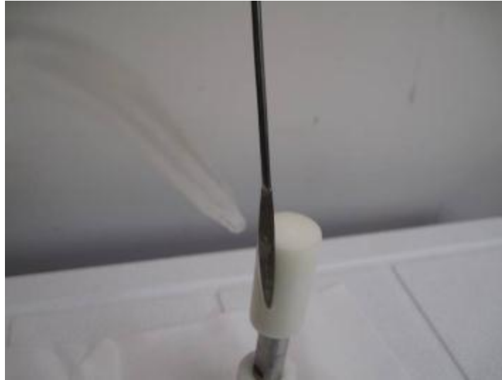
Figure 3.17: Separating sleeve from mandrel using spatula and alcohol
