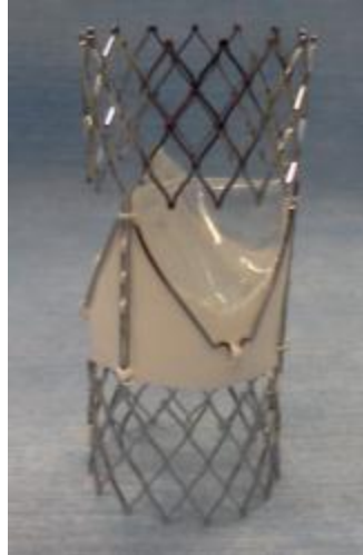
Figure 4.12: Sutured Crown Stent 1 - view 1
