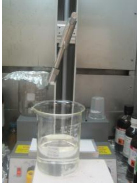
Figure 2.35: Mandrel in Dipping Position
