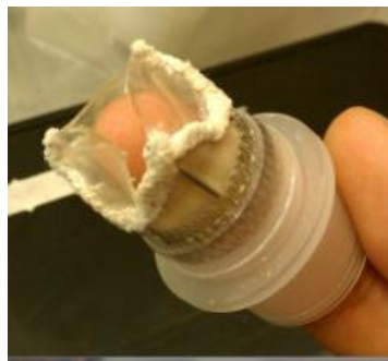
Figure 4.14: Valve rupture in cycle tester
