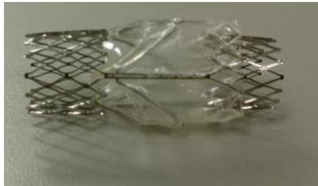
Figure 4.8: Post collapsed thermoformed Crown Stent 1 - view 1
