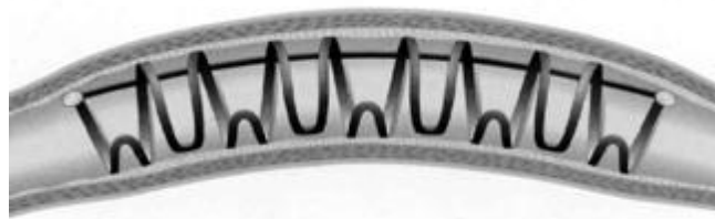
Figure 2.3: Stent Formed From Stainless Steel Sheet, Featuring an Axial Backbone with Integral Gold Markers (Stoeckel, Bonsignore, & Duda, 2002)
