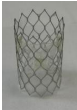
Figure 3.1: Generic Curved after dip casting leaflet
