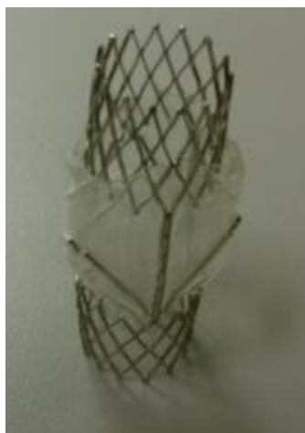
Figure 4.9: Post collapsed thermoformed Crown Stent 1 - view 2
