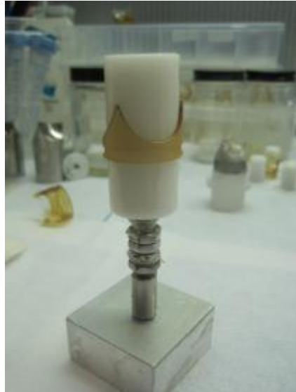
Figure 3.15: Polyurethane stent placed on exterior sleeve mandrel
