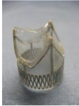
Figure 3.3: Generic Crown after dip casting valve leaflet
