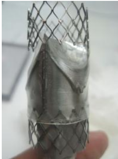
Figure 3.20: External sleeve on stent and aligned with mandrel commissure tips
