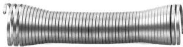
Figure 2.5: Coil Stent Fabricated from Nitinol Ribbon (Stoeckel, Bonsignore, & Duda, 2002)
