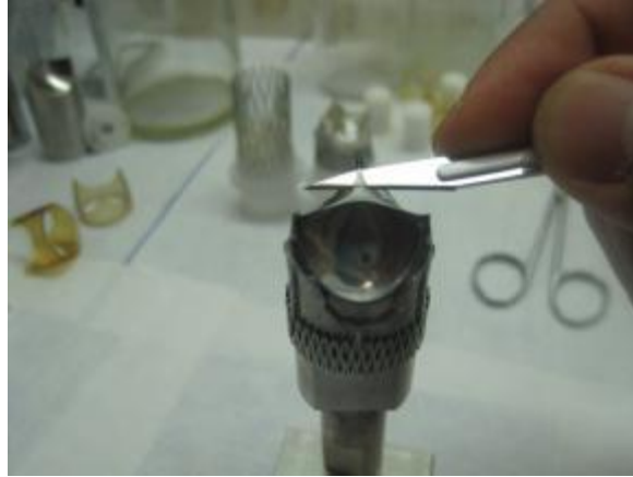
Figure 3.12: Trimming cured Angioflex™ off the top flat surface on the mandrel
