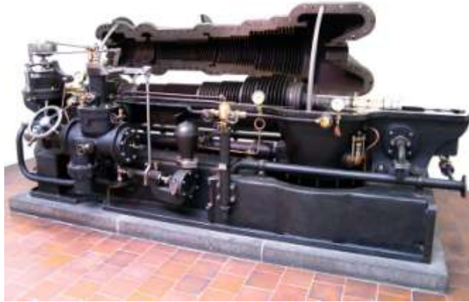
Figure 1-3 - Conventional steam turbine
