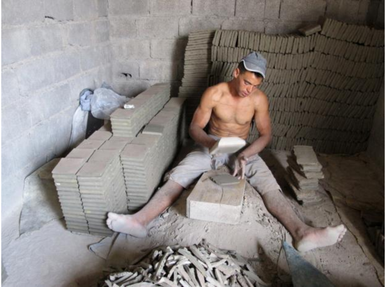
Figure 3: An artisan pounds a tile into shape. Note the pile of tile edges in front of the artisan.
