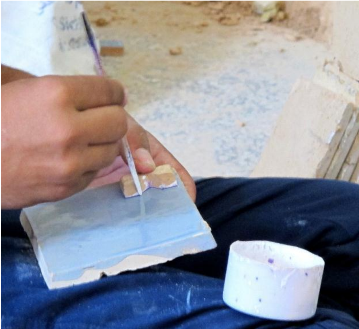
Figure 14: An artisan traces the shape of a zillij tile onto a tile to be cut.
