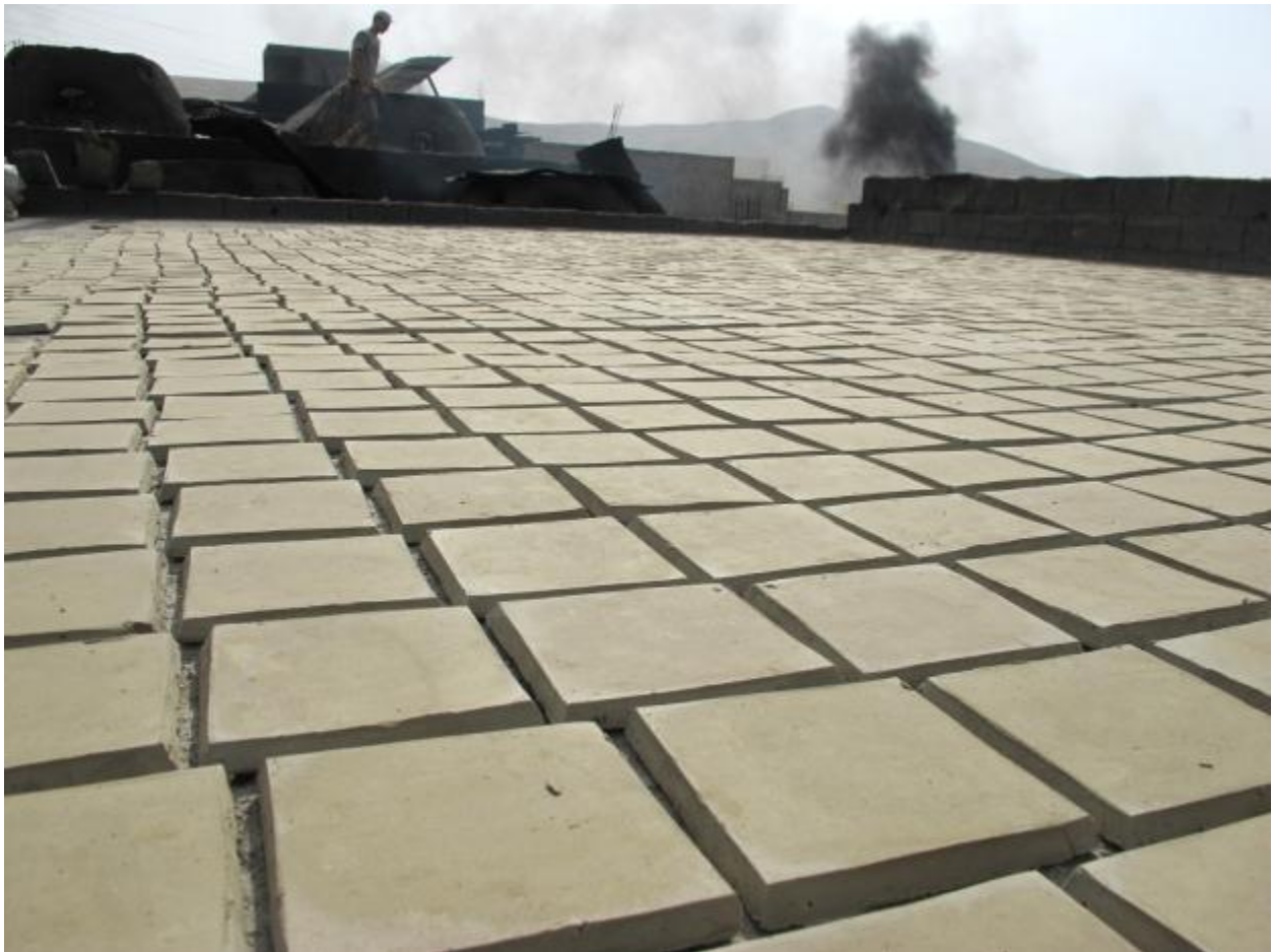
Figure 4: Tiles dry in the sun on the roof of the kiln facility.
