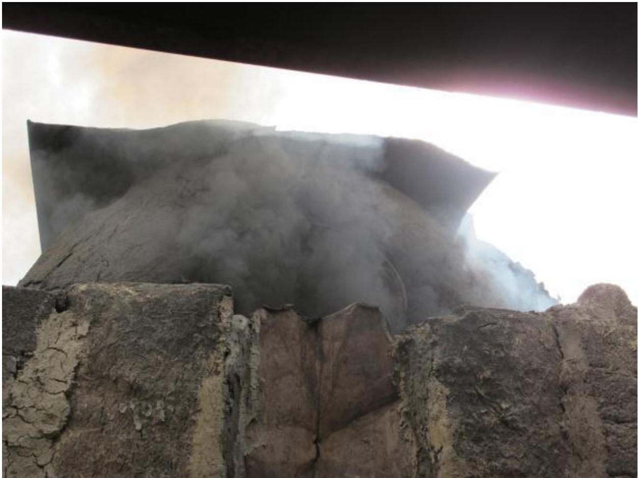
Figure 12: The kiln, sealed with clay and sheet metal, is in use.
