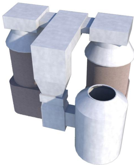
Figure 22: A rendering of the ducting connecting the scrubber to the two kilns.
