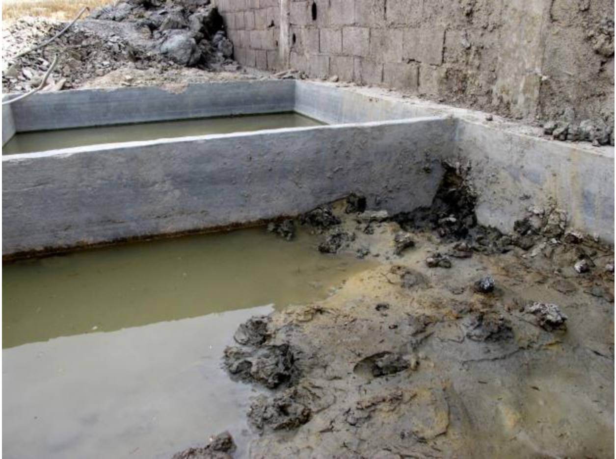
Figure 2: Water is added to the clay so that the clay is soft enough to work with.
