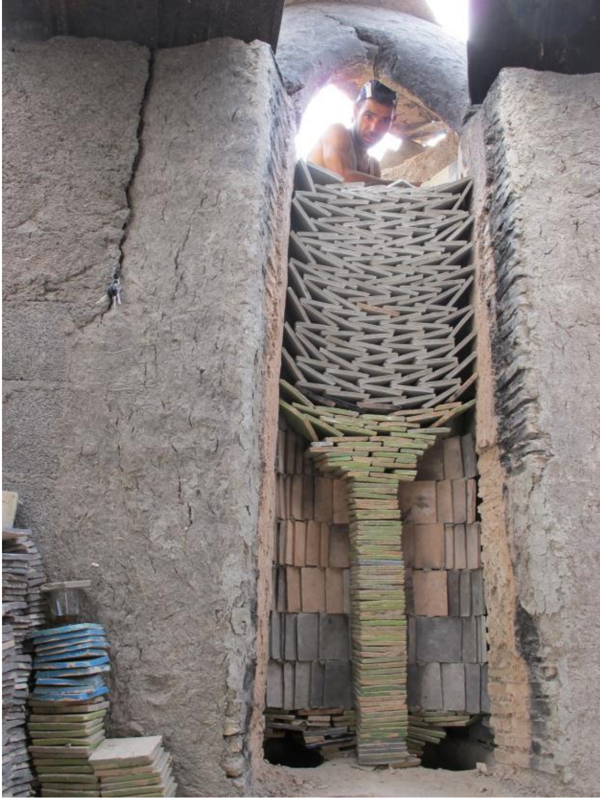
Figure 11: An artisan stacks tiles inside of a kiln to be fired.
