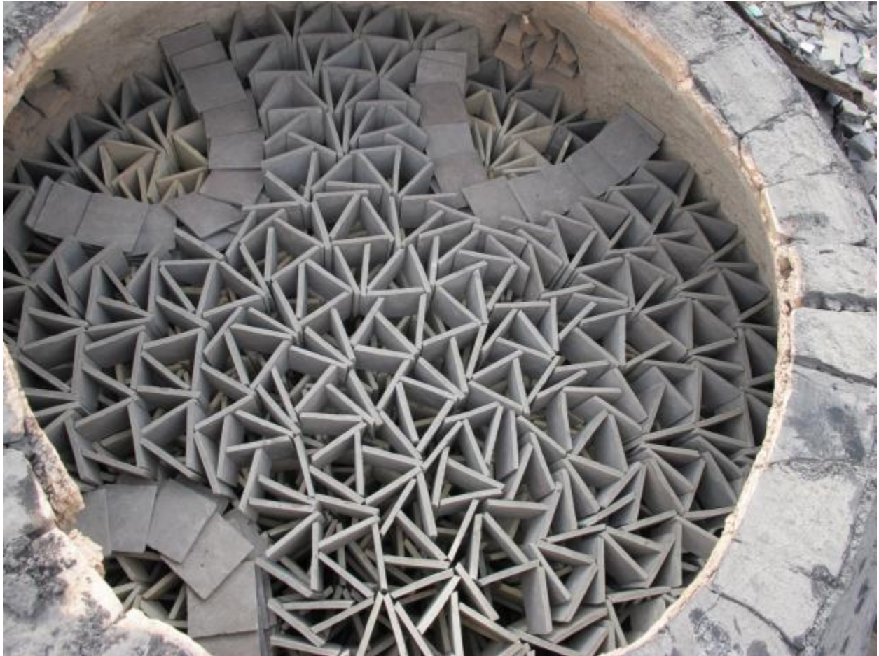
Figure 10: Tiles stacked in a kiln ready to be fired (Viewed from the top of the kiln).
