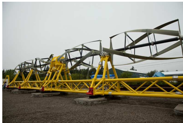
Figure 4.13: An Underwater Turbine in Cobscook Bay[127]
