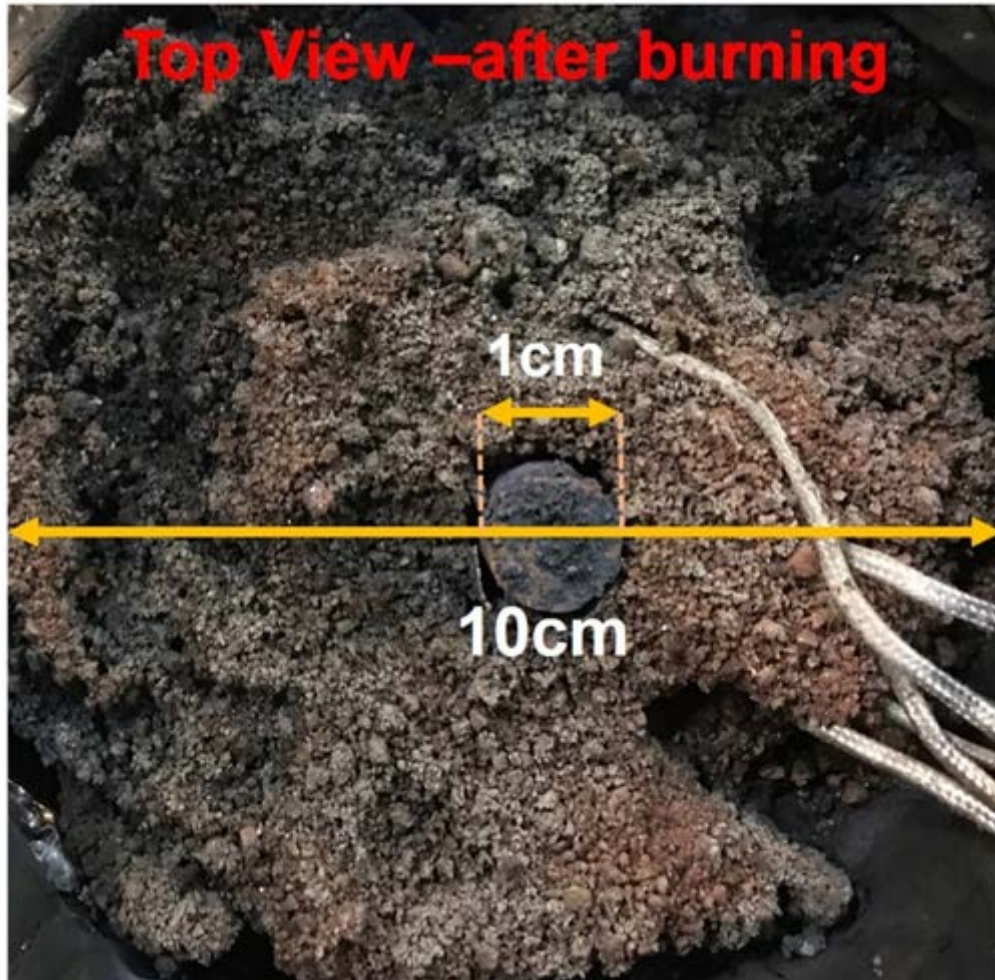
Figure 21: Top view of burnt fuel at 25 kW/m 2 heat flux
