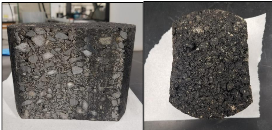
Figure 3: Photographs of the asphalt disks used in the MMLS.
