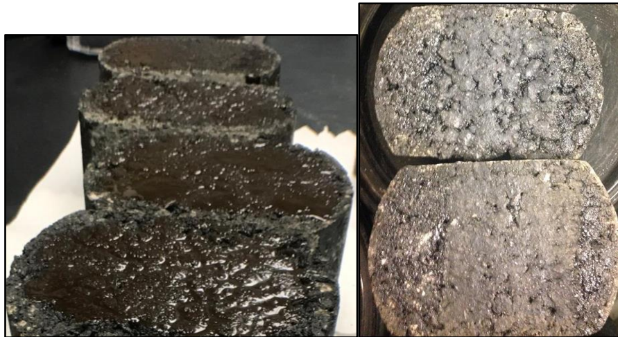
Figure 9: Asphalt-Based Rejuvenator Run. Left is a Photograph of the Pavement Samples Before MMLS. Right is a Photograph of the Pavement Samples after MMLS.
