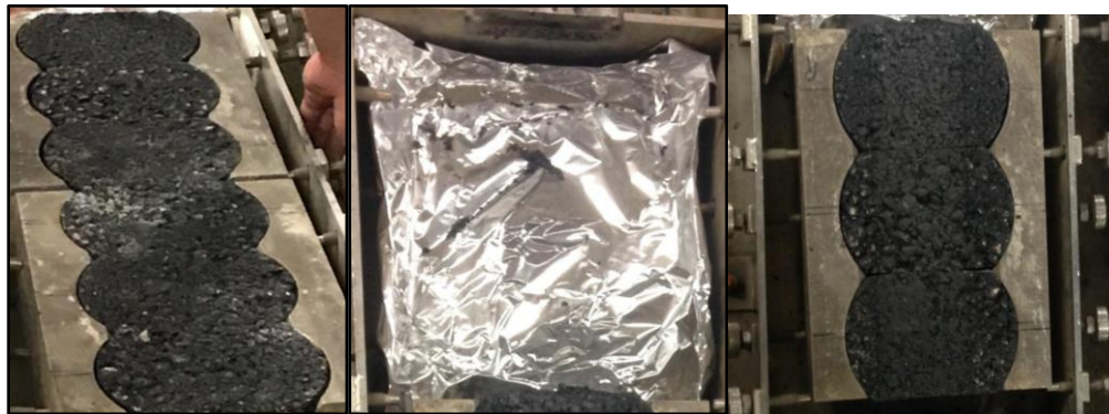
Figure 8: Second Control Run. Left is a Photograph of the Pavement Samples Before MMLS. Middle Image is Particulate Detached During the Testing. Right is a Photograph of the Pavement Samples after MMLS.
