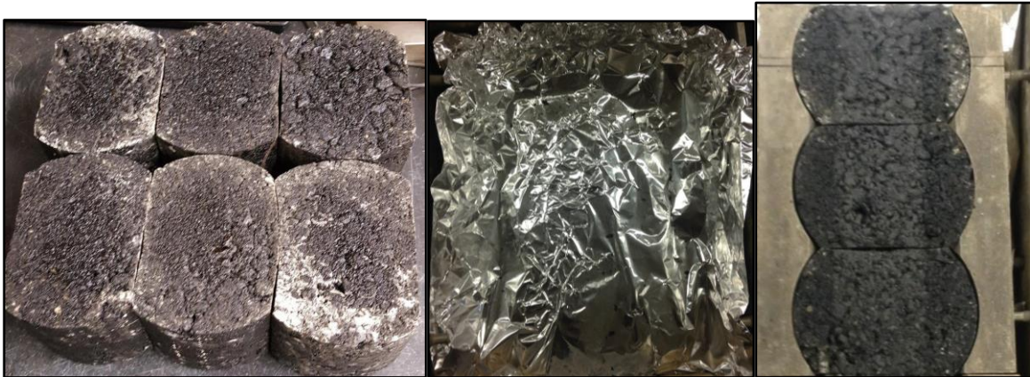
Figure 10: Bio-Based Rejuvenator Run. Left is a Photograph of the Pavement Samples Before MMLS. Middle Image is Particulate Detached During the Testing. Right is a Photograph of the Pavement Samples after MMLS.
