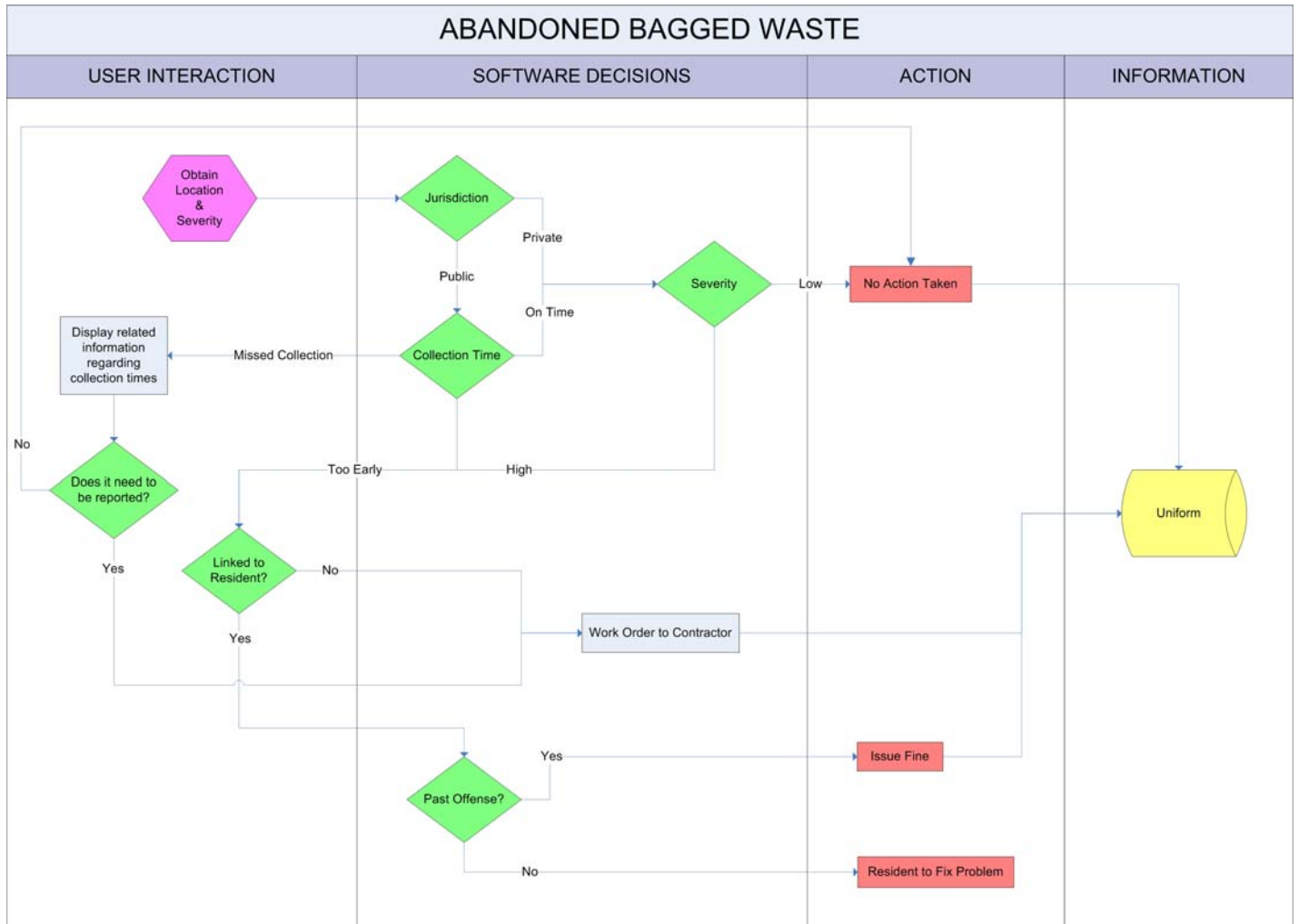
Figure 56 - Abandoned Bagged Waste Flow Diagram for Software Implementation
