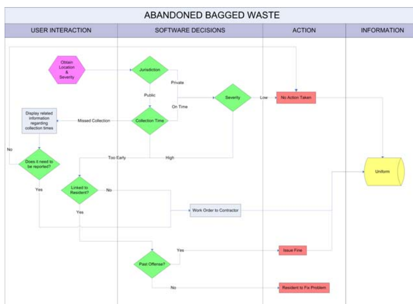
Figure 5 - Software Flow Diagram Specifications
