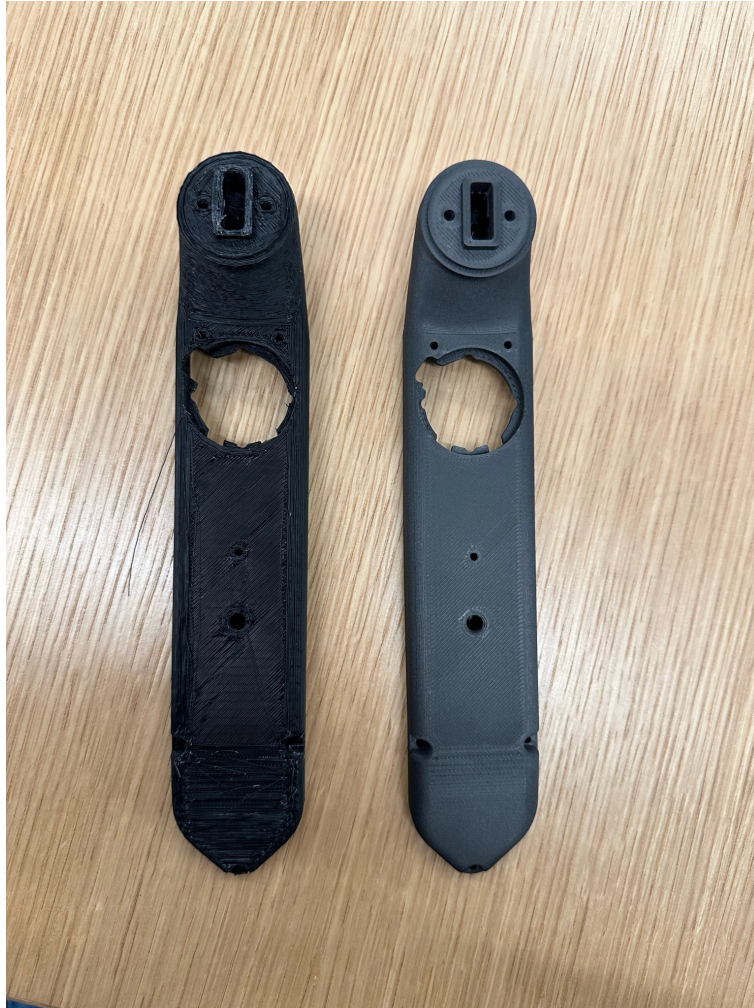
Figure 2: Comparison of ABS (left) and Onyx (right) prints
