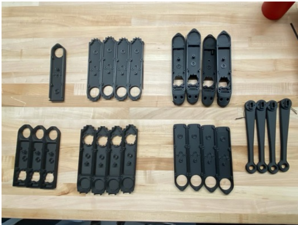
Figure 12: Actuator Module Shells printed in Onyx
