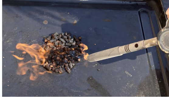
Figure 3.2. ANS burnable pellets being ignited by the propane blowtorch
