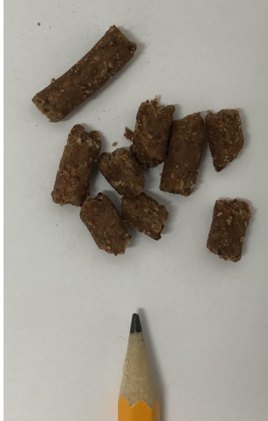
Figure 3.1. Argan burnable pellets made from post-cracking crumbs fed and extruded through the oil extrusion machine
