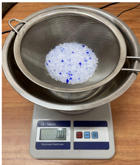
Figure 3.5. Testing setup for the silica gel cat litter absorbency pouring trials
