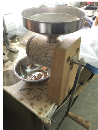
Figure 3.4. Manual grinding machine used to make the ANS pebbles and ANS powder
