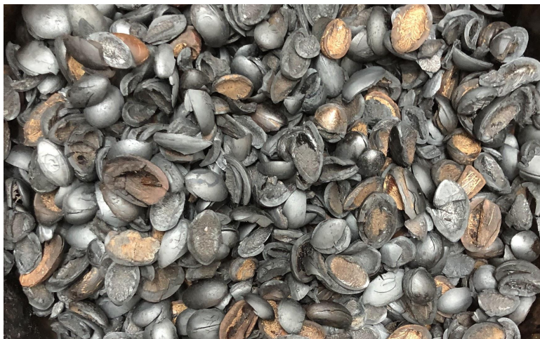
Figure 3.6. ANS shells after being cooked in a lidded pot for 7 hours to make charcoal
