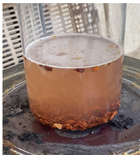
Figure 3.7. Crushed ANS being boiled in sodium hydroxide solution in an attempt to extract cellulose fibers
