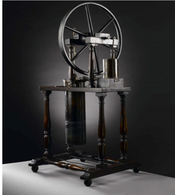
Figure 5: Model of Stirling engine at the National Museum of Scotland (Linda Hall Library, 2019)
