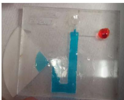
Figure 72: Paper Based Pump 2.26 during Testing
