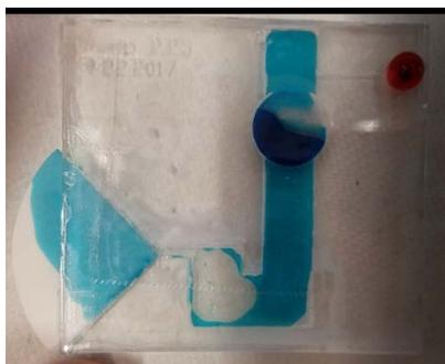
Figure 70: Paper Based Pump 2.25 during Testing
