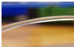
Figure 92: Droplets Formed in Tube from Weight Driven Pump
