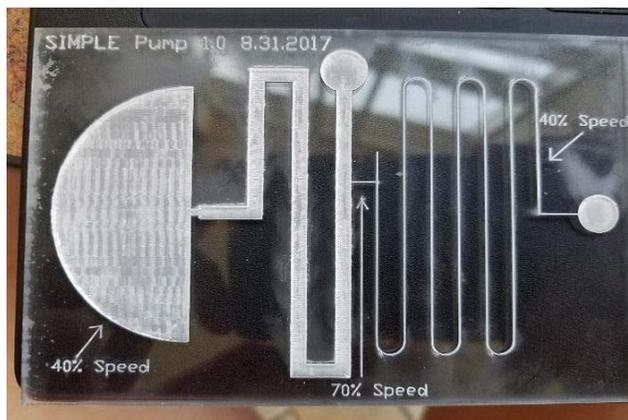
Figure 45: Photograph of Paper Based Pump 1.0 The chip size is about 57x38x3 mm
