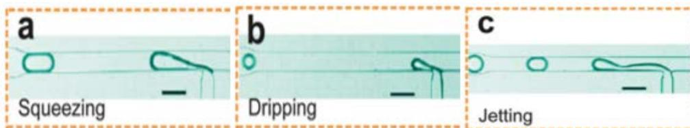
Figure 11: Photographs of Droplets in the Squeezing, Dripping, and Jetting Regimes [30]
