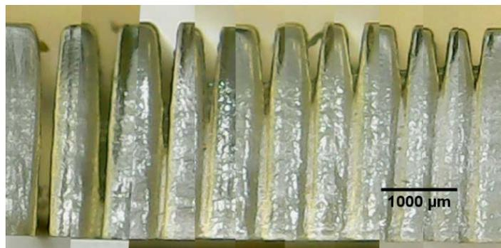
Figure 16: Vector Cutting Increasing Speed
