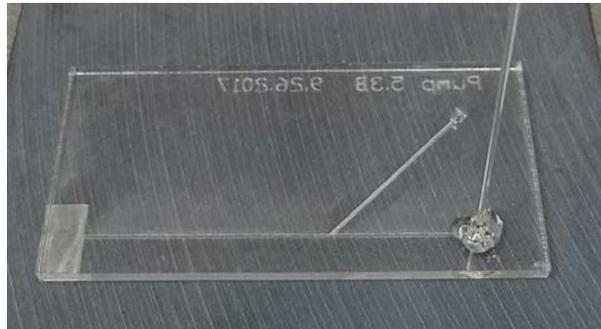
*Figure 77: Photograph of Gravity Driven Pump 5.3 with Borosilicate Tube Attached Via UV Hardened Glue*
