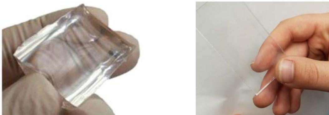
*Figure 1 a (left) Photograph of PDMS [5]. 1 b (right) Photograph of Acrylic*
