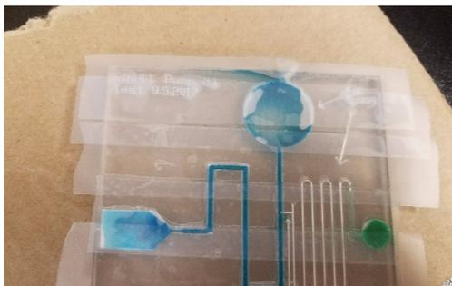
Figure 50: Photograph of Paper Based Pump 2.1 Sealed with Scotch Tape
