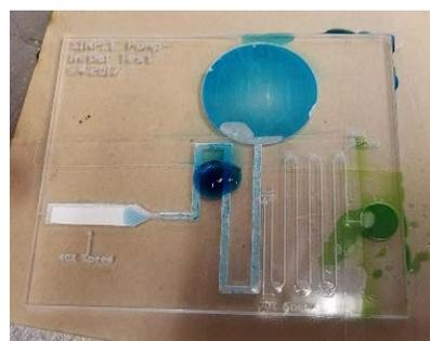
Figure 87: Paper Based Pump with Leakage
