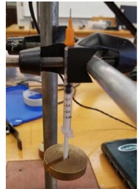
Figure 79: Setup of Experiment to Measure Frictional Force in a Syringe
