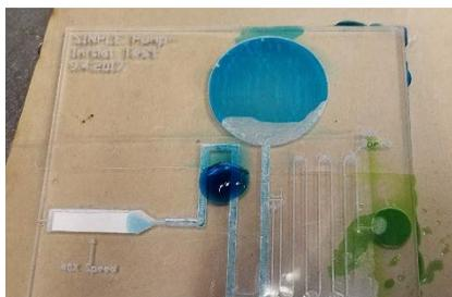
Figure 47: Photograph of Paper Based Pump 2.0 with Leakage
