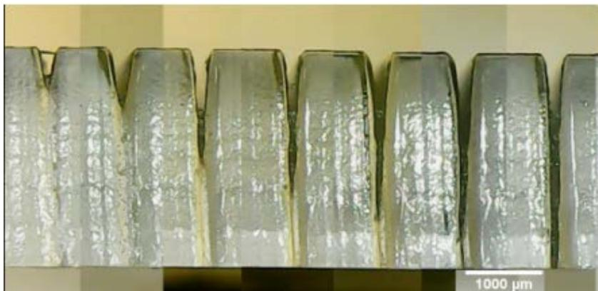
Figure 22: Vector Engraving Increasing Number of Passes
