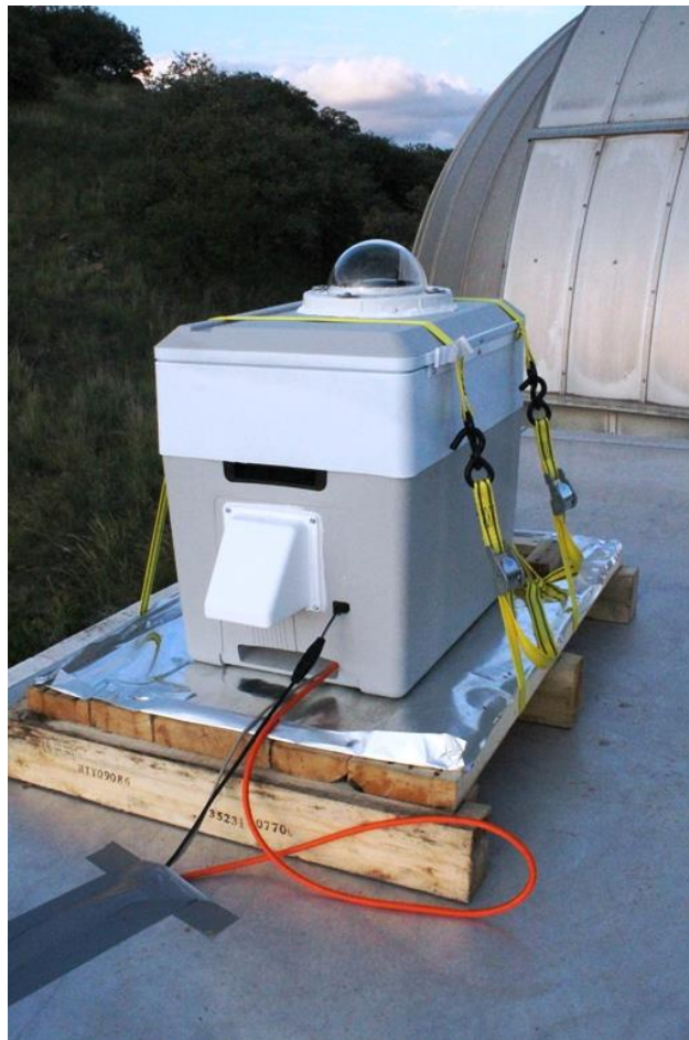
Figure 1.1: All-sky-imager prototype for the MANGO remote system
