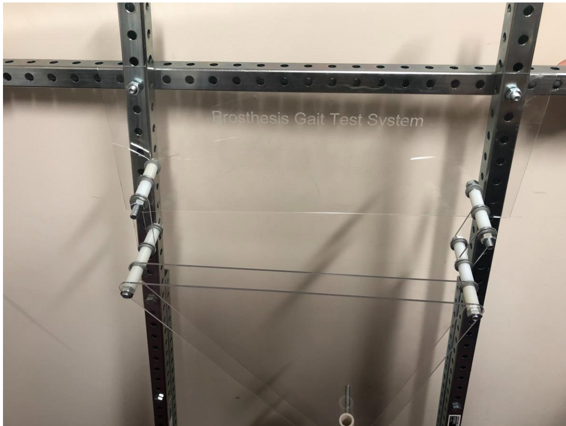
Figure 44: Acrylic-Cut Linkage System for Gait Analysis
