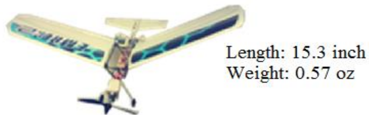
Figure 5: Parkzone ® Ember modified with articulated wings
