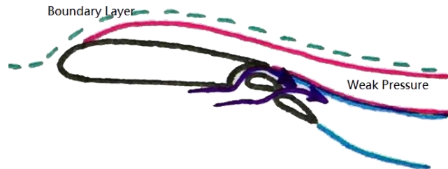
Figure 32: Section view of fowler flaps
