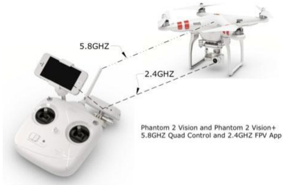
Figure 101: 2.4GHz/5.8GHz frequency wireless communication structure
