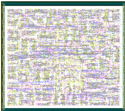
Figure 3.9: Layout of the decoder core area.
