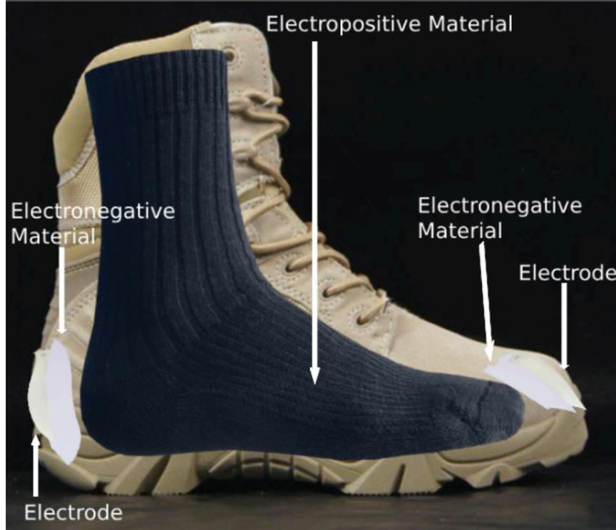
Figure 8. Heel Toe Boot TENG design [13].
