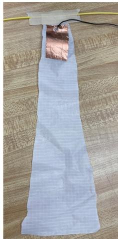
Figure 65. Inverted triangle structured TENG (flapper).
