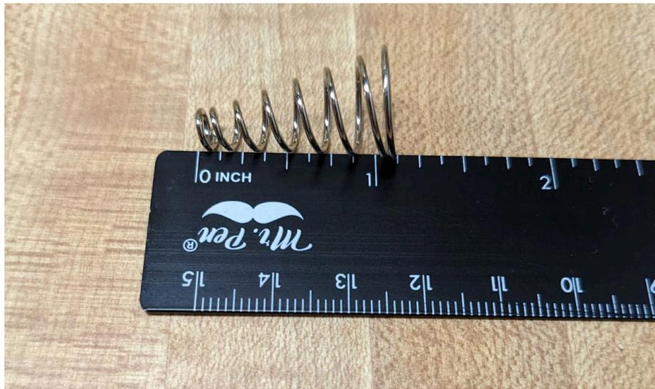
Figure 57. Conical springs used in attempts to increase TENG power output.
