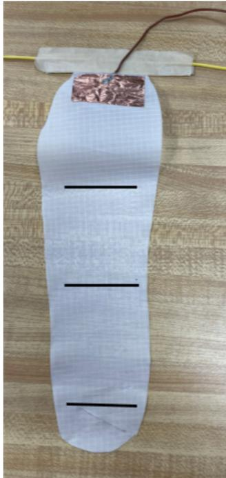
Figure 63. Three slit structured TENG (flapper).
