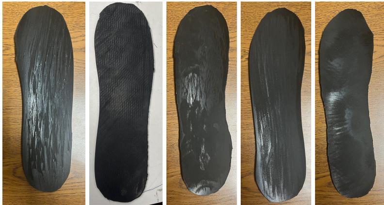
Figure 52. The textured insole. From left to right, the insoles are the deep score, the shallow score, the dremel, the clay cutter, and the cheese grater textures.
