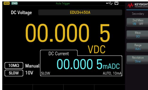
Figure 29. The DMM interface while measuring both voltage and current [31].
