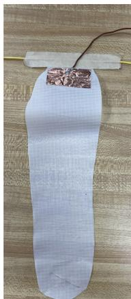
Figure 61. Baseline structure for the TENG (flapper).
