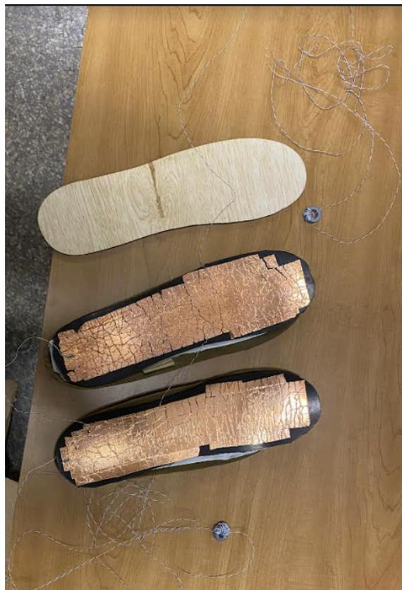
Figure 50. The wooden pattern and examples of the insole shaped TENGs.
