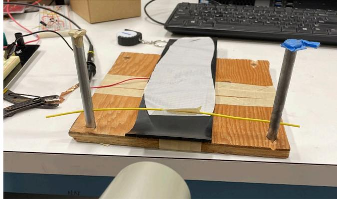
Figure 59. Wind TENG Testing setup.
