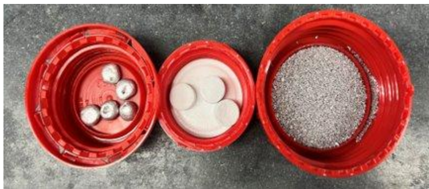
Figure 2: From left to right the alumina pellets, the aluminum hydride tablets, and the aluminum granules.
