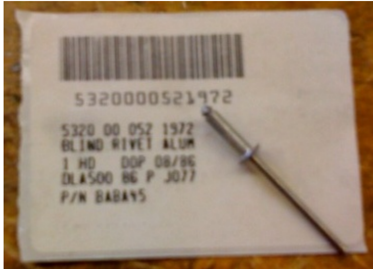
Figure 79: Photo of rivet being used on the Impact Attenuator structure
