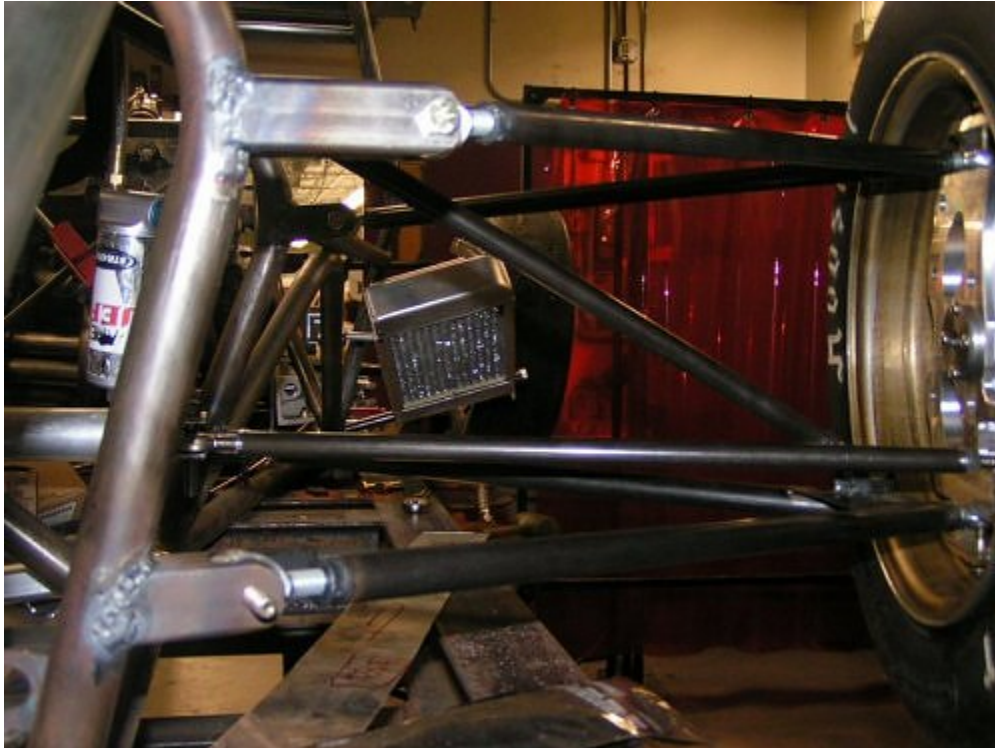
Figure 1: Excessive Tab Length on 2007 WPI Chassis
