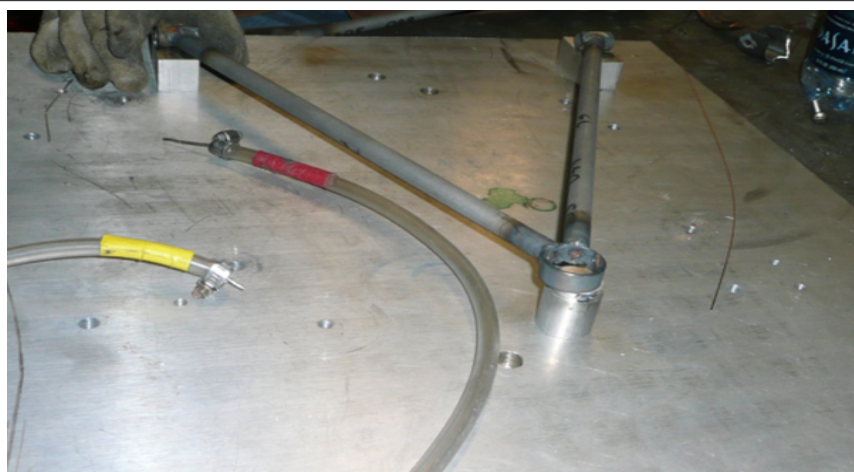
Figure 37: Control Arm Fabrication Jig
