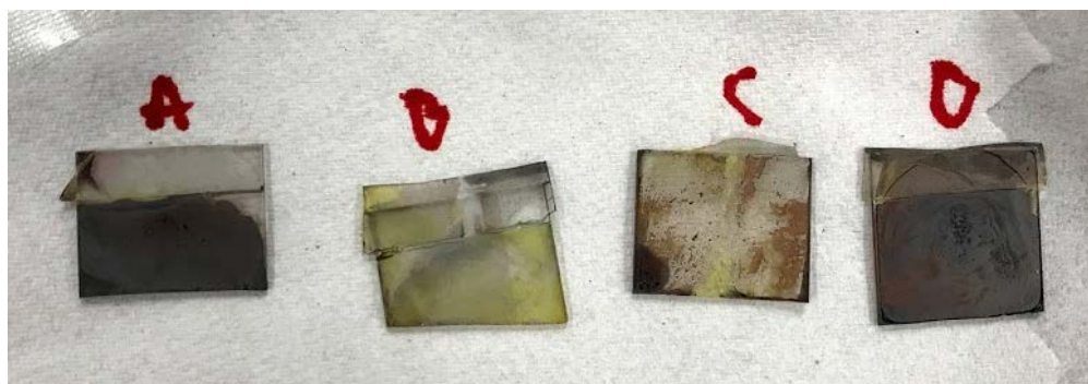
Figure 22. The first \text{MaPbI}_3 layers obtained. Sample A an old dip coating solution that initially worked. Samples B and C using a solution mixed that day. Sample D had the same parameters as B and C but was dipped in the old dip coating solution.
