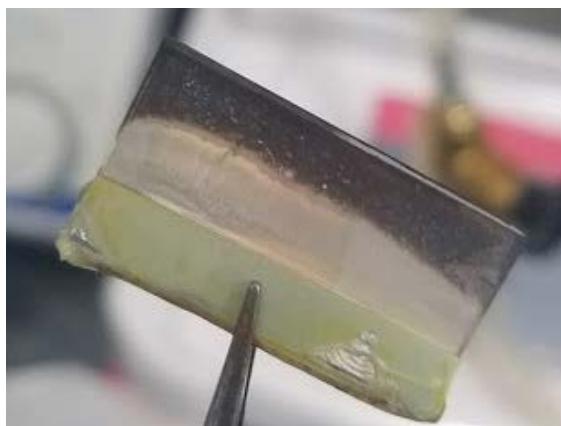
Figure 23. Example of tape contamination after dip coating and annealing.
