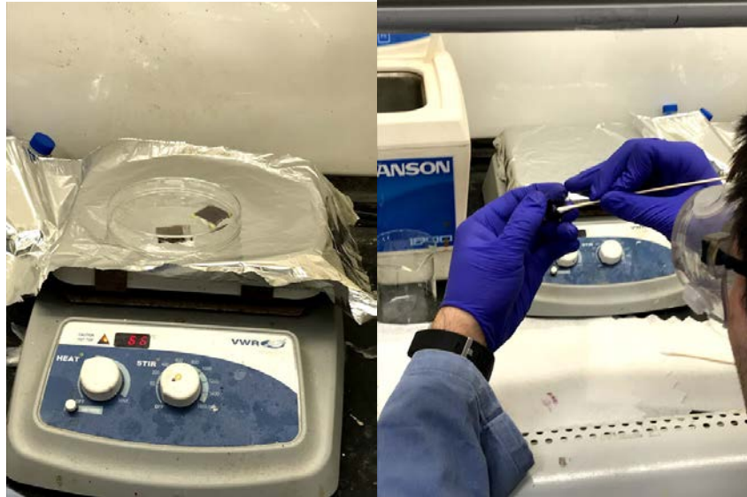
Figure 49. Solar cell processing in the fume hood of annealing CuSCN and wiping the contact for the ITO conductor.
