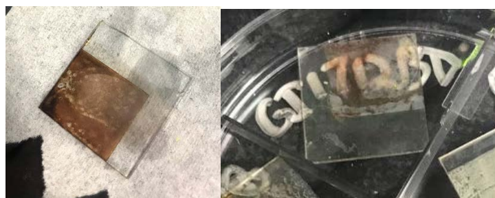
Figure 20. (Left) FAPbI 3 dip coating layer just after dipping. (Right) Same layer after sitting in the glovebox.
