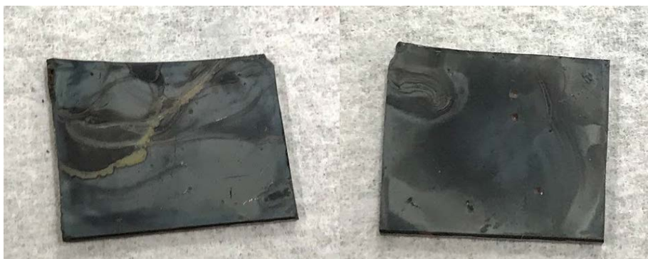
Figure 26. MAPbI 3 layers after layer processing. (Left) Lines left in the processed layer from drying. (Right) Sample dried flat without drying lines.
