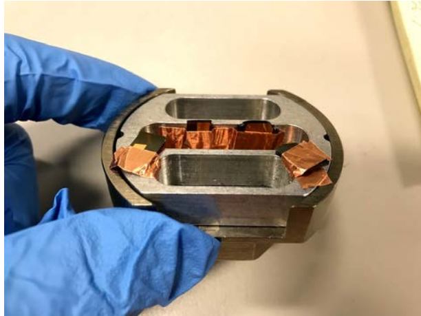
Figure 12. Examples of SEM holder mounting with samples attached.
