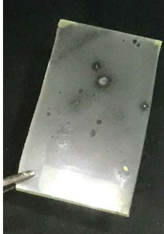
Figure 24. Example of precipitates in the PbI_2 spin coating step.
