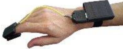
**Figure 10: AliveTec wrist-style wireless pulse oximeter<sup>18</sup>**
