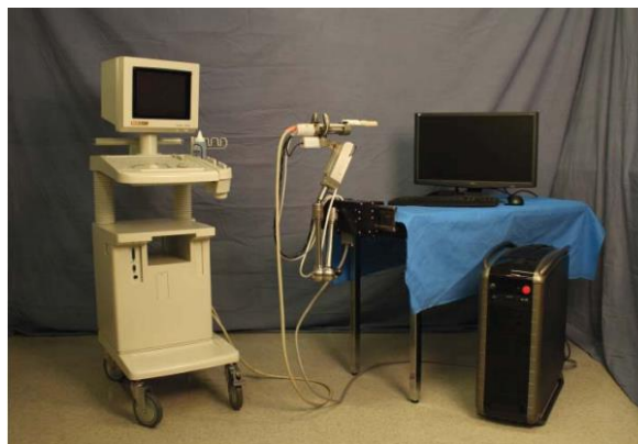
Figure 1. 2: A robot for manipulating a transrectal ultrasound probe for image-guided prostate intervention [7]
