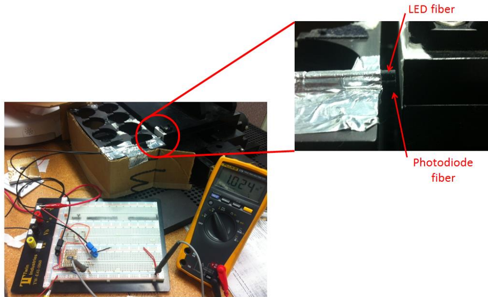
Figure 4. 6: LED and photodiode test
