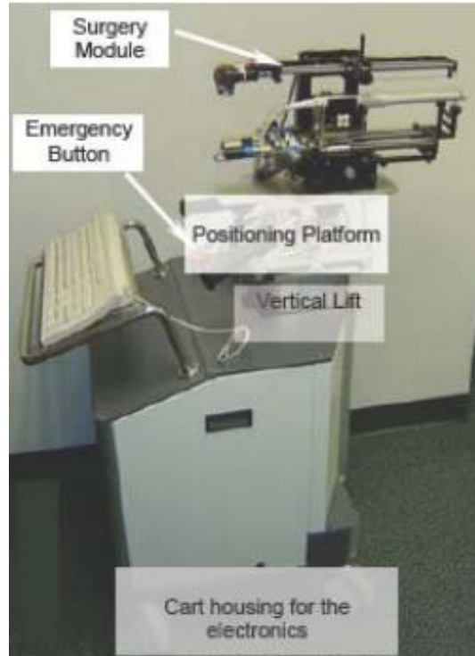
Figure 1. 10: A 16-DOF system for prostate brachytherapy [15]
