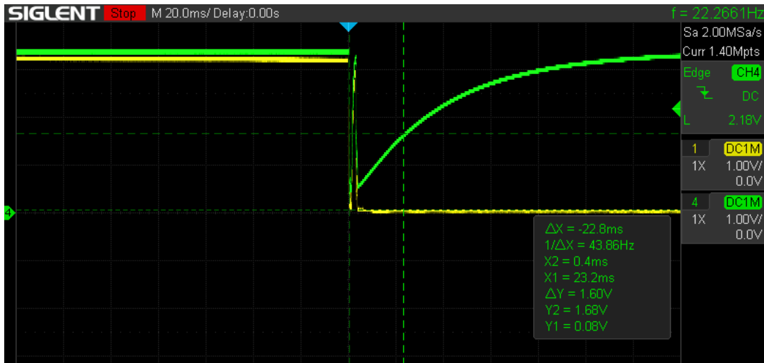
Figure 30: Monostable input (yellow trace) and output (green trace).
