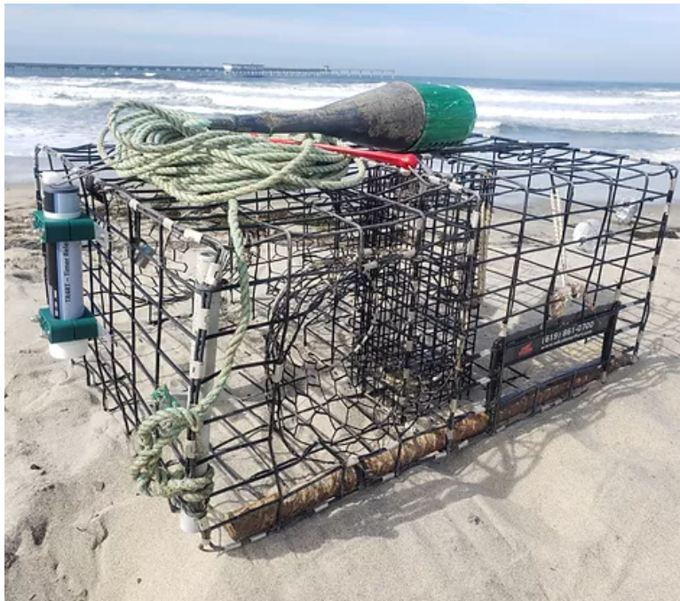
Figure 7: SubSea Sonics TR4RT attached to a single trap with rope and buoy stowed on top [28].
