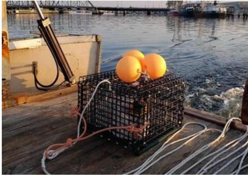
Figure 5: EdgeTech 5112 system installed on a lobster trap cage [24].
