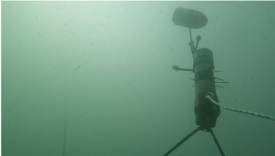
Figure 38: Lobster R.O.L. deployed in 45 feet of water.
