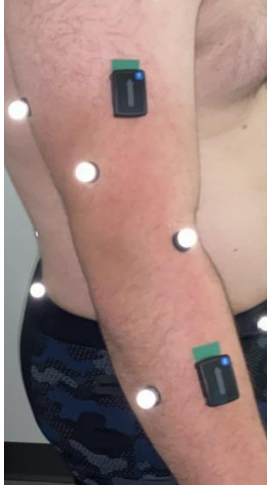
Figure 11: Typical Delsys accelerometer placement on the forearm and bicep of a participant.
