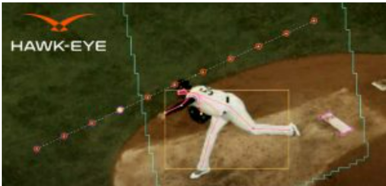
Figure 12: Breakdown of Hawkeye Motion Capture working by calculating estimated joint centers of the pitcher (Sony, 2020).
