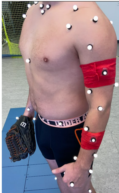
Figure 43: Example of markerset placement on WPI pitcher with increased number of markers on pitching arm.
