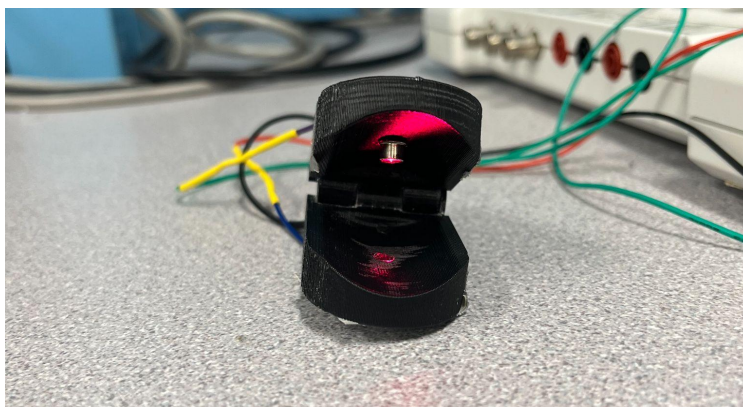
Figure 5.4 - Photograph of model printed in ABS with implanted components.
