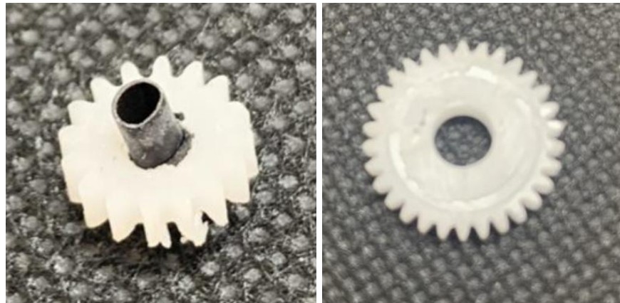
Figure 68: 4:3 Gear Train Fatigue Results.
