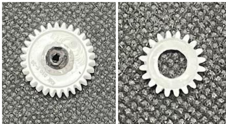
Figure 69: 16:30 Gear Train Fatigue Results.
