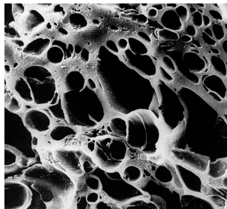
Figure 3: Electron microscope image of an activated carbon structure (Activated Carbon Pore Structure).
