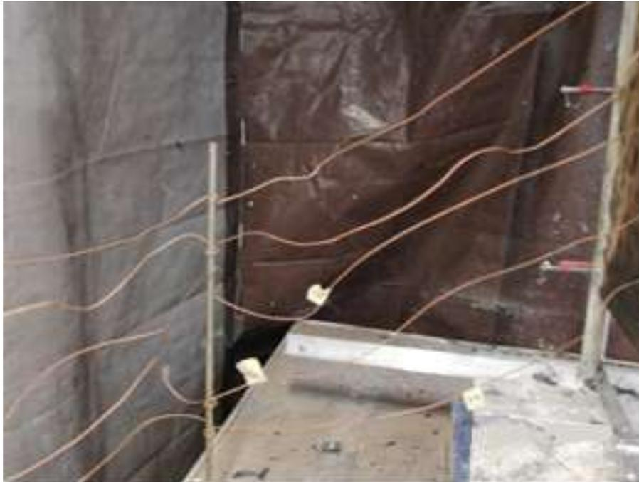
**Figure 10: Thermocouples attached to the cardboard**
