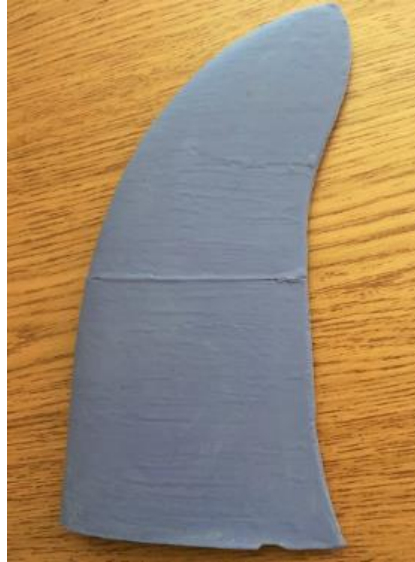
Figure 82: Shore A Harness 45 silicone flexible flipper
