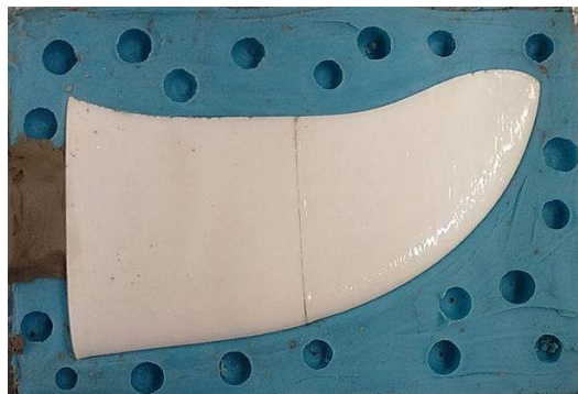
Figure 81: Silicone master mold of flipper with 3D printed part inside
