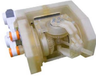
Figure 18: Ball and socket mechanism prototype [32] 7
