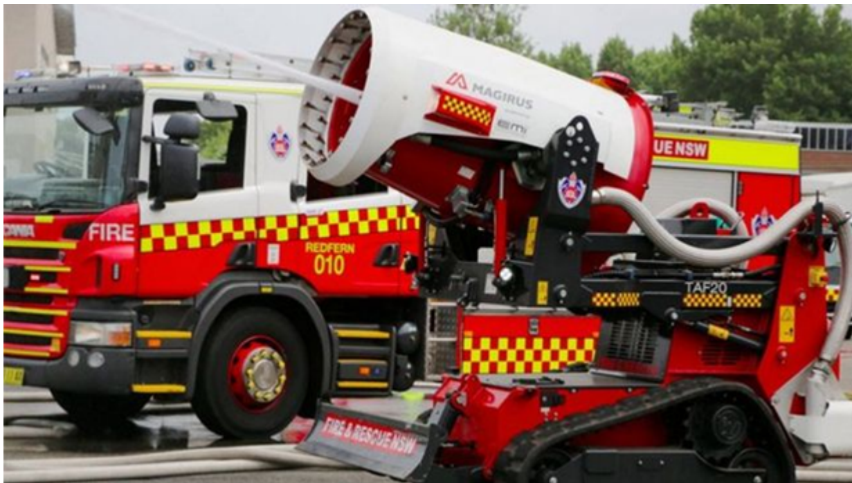
Figure 1. The TAF20 firefighting robot testing its water cannon. Notice the plow on the front of the tractor and the focused stream of water (Bharat, 2015).
