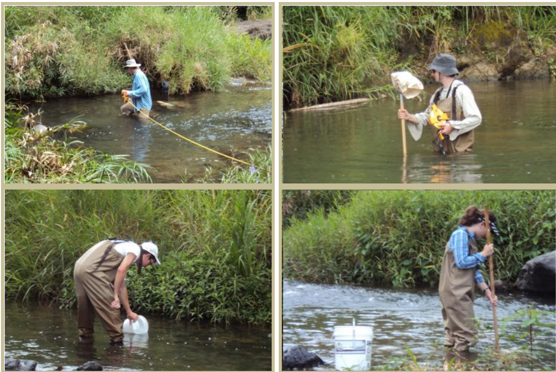
Figure 7: (Clockwise from top left): Team member determining ACW, assessing physical features, kick sampling, collecting water samples
