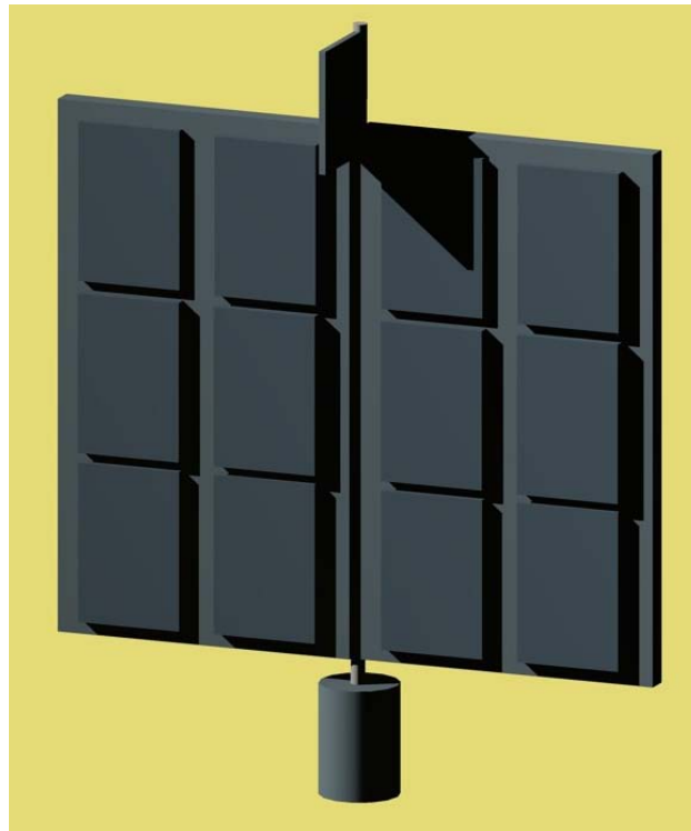
Figure 3: Auxiliary Bifacial Solar Tracker
