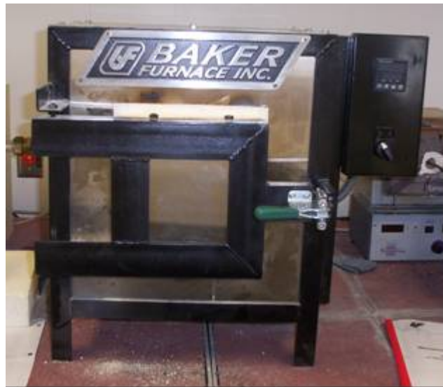
Figure 3-2: Baker Model 6 lab Furnace with Honeywell Temperature Control
