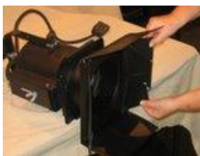
Figure 46: Fresnel with barn door (open)
