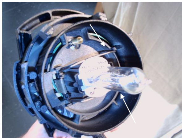
Figure 22: Brass holders, where to pinch to remove
