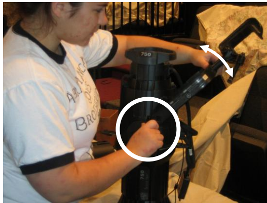
Figure 11: "Yoke locking knob" on an ellipsoidal
