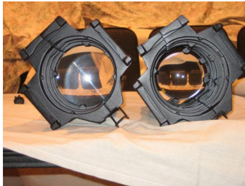
Figure 40: A 50° and a 36° barrel side by side.
