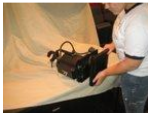
Figure 44: Fresnel with barn door (closed)
