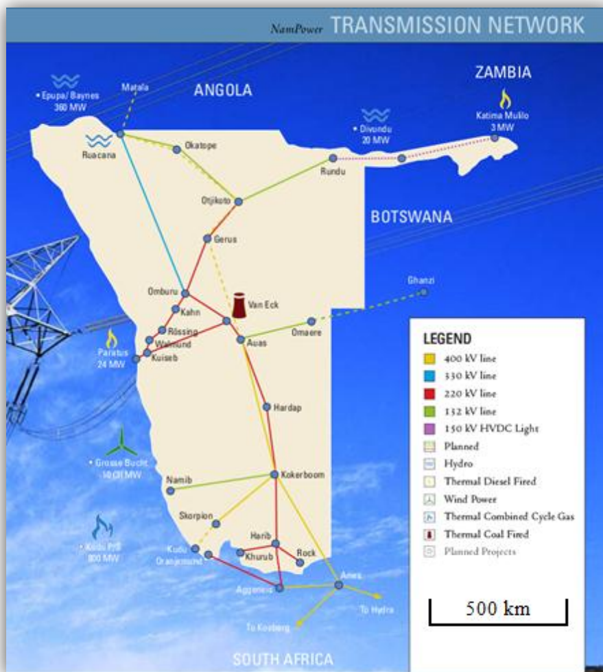
Figure 1: NamPower transmission lines and power distribution (NamPower, 2009)
