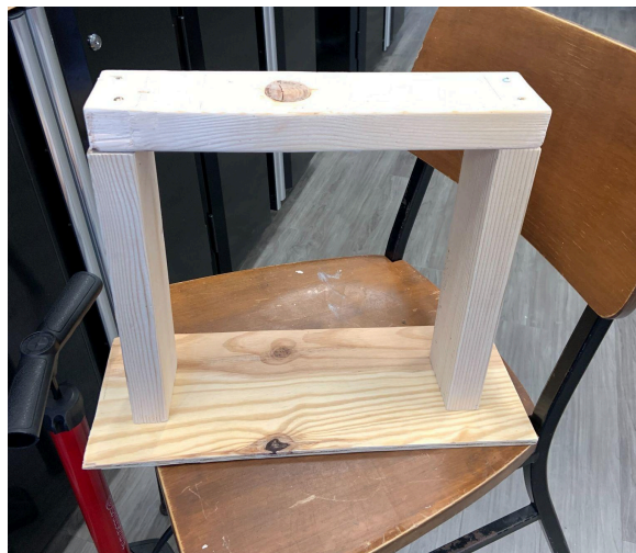
Figure 23. Wooden frame used in elderly adult human testing to simulate the slider being adhered to the bottom of a cabinet.
