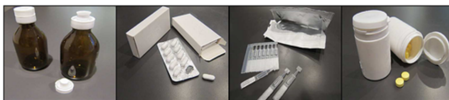
Figure 1. Four types of packages in the study. From left to right: glass bottle with screw cap, pill plate, disposable plastic dropper, and plastic jar with hinge cap (Sormunen et al., 2014).
