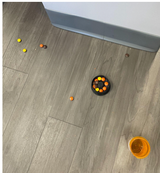
Figure 32. Result of drop test trial on linoleum floor at shelf height (30.5 inches).
