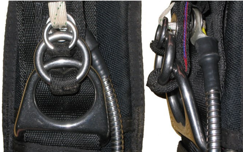
Figure 62: 3-Ring Release Mechanism used in Skydiving [67]
