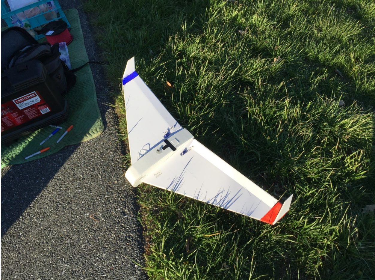
Figure 64: Final Glider Ready for Balloon Testing
