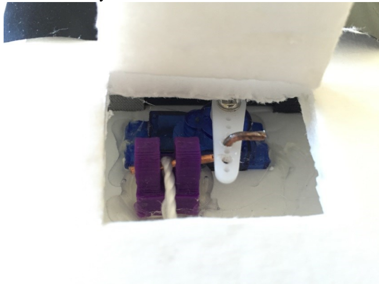
Figure 63: Final Release Mechanism
