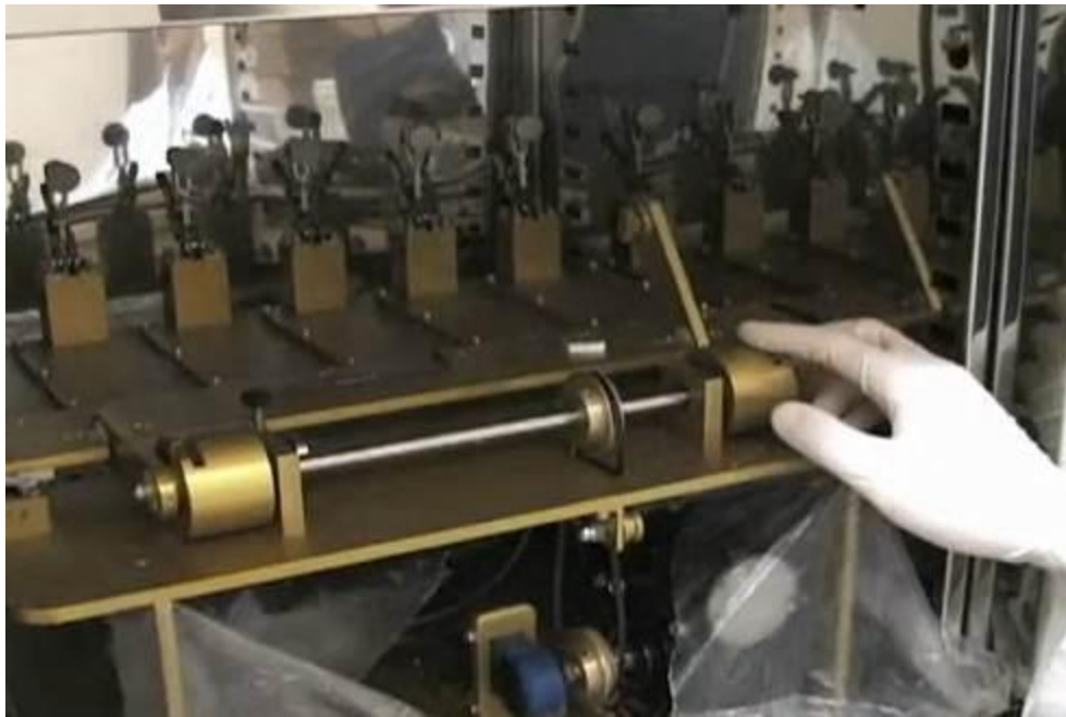
Figure 8. University of California-Berkley custom-built uniaxial stretch device (Reprinted with permission)
