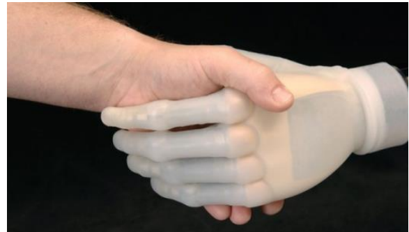
Figure 4b: i-limb with plastic covering [17]
