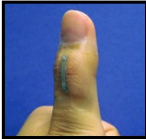
Figure 8: A sensor based on silver nanowires is mounted onto a thumb joint [21].
