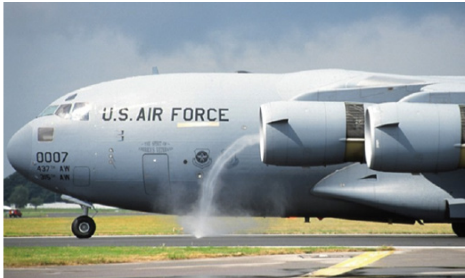
Figure 1.1 Ground vortex on a military turboprop engine visible due to water condensation inside core (Shmilovich and Yadlin, 2011).
