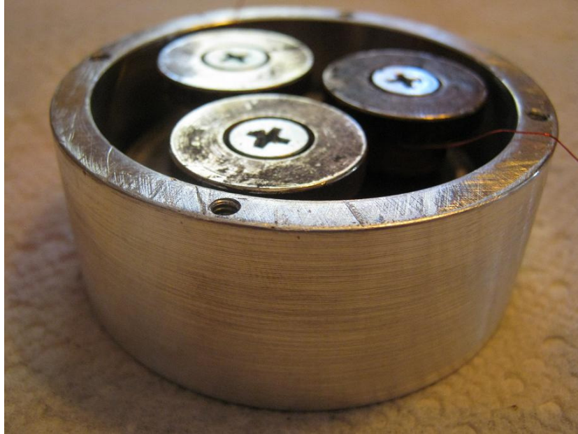
Figure 7.2-3 – Experiment 4 Stator. This figure shows a picture of the stator used for experiment 4. Note the large distance between the top of the stator poles to the top of the stator case.
