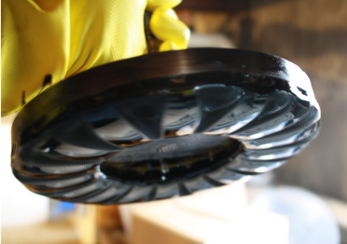
Figure 5.2-7 – Experiment 2, Rotor, Post-Test. This figure shows Experiment 2’s rotor after the test. Note the ferrofluid magnetically attached to the permanent magnets, with the magnetic forces exceeding the gravitational forces. This highlights the need for a containment tank, a lesson learned that was incorporated into experiments 3 and 4.
