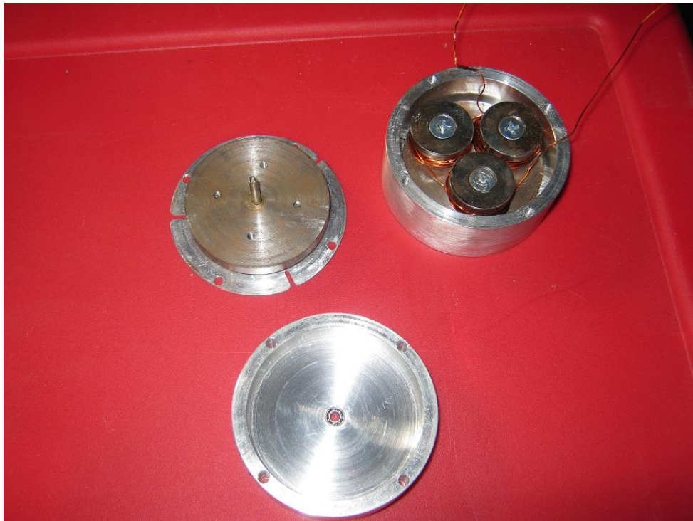
Figure 6.2-2 – Experiment 3 Generator. This figure shows pictures of the generator used for experiment 3, a 2” diameter axial flux PMM.
