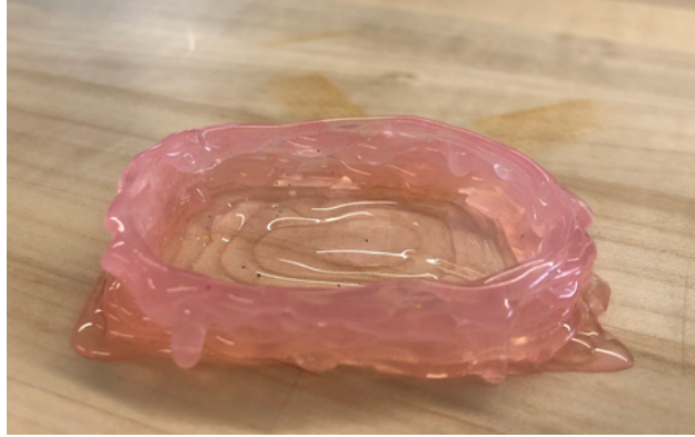
Figure 28: Layers of silicone printed by hand without pooling
