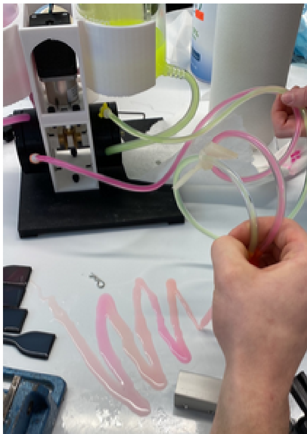
Figure 27: Duty cycle of each peristaltic pump shown with dye
