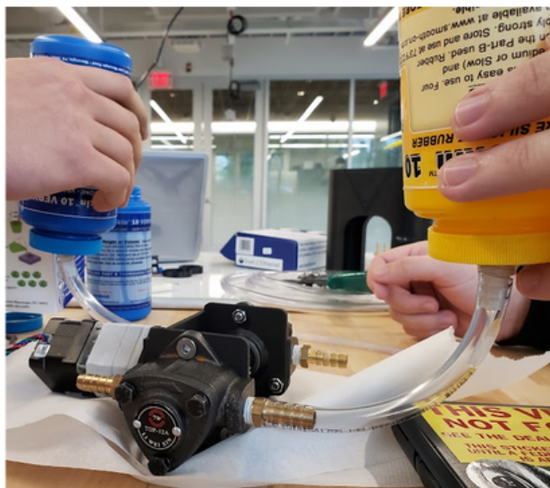
Figure 19: Testing two gear pumps with Dragon Skin 10 VF
