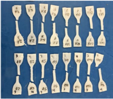
Figure 16: Broken Dragon Skin 10 VF samples after tensile testing.
