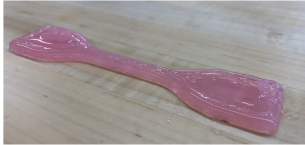
Figure 31: Dogbone sample printed on the E3D
