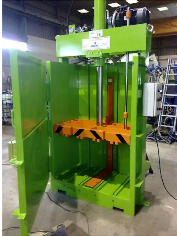
Figure 12. Image of a potential design: A vertical hydraulic baling press. xv
