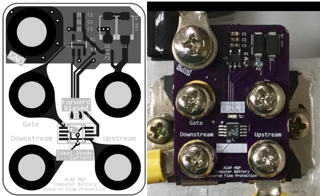
Figures C7 and C8: Ideal Diode board layout; Ideal Diode circuit
