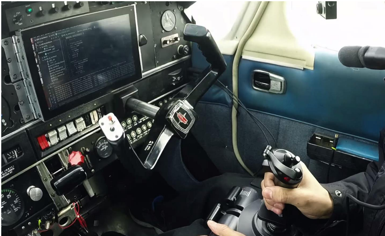
Figure C9: Fly-by-wire taxiing demonstration
