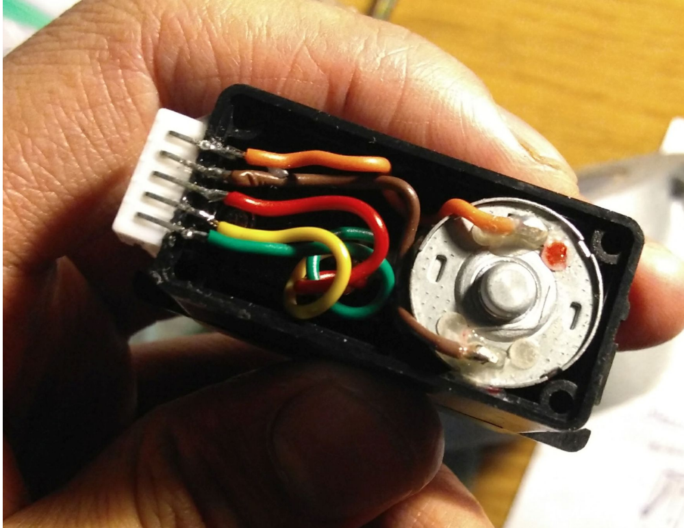
Figure D.10: Modified clutch servo motor. The rear cap was removed to show the wiring
