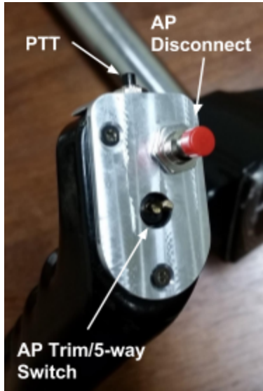
Figure B9: Yoke Switches
