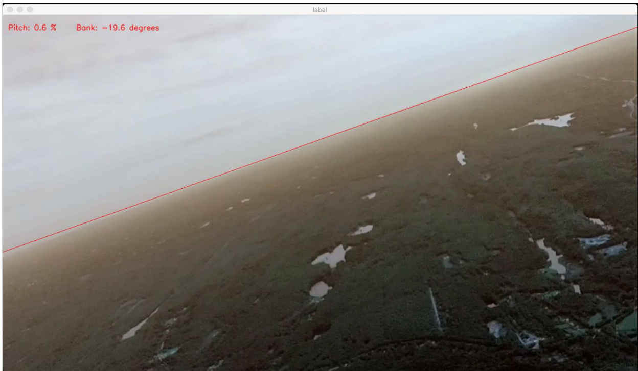
Figure 16: The calculated horizon line superimposed in red onto the input image.
