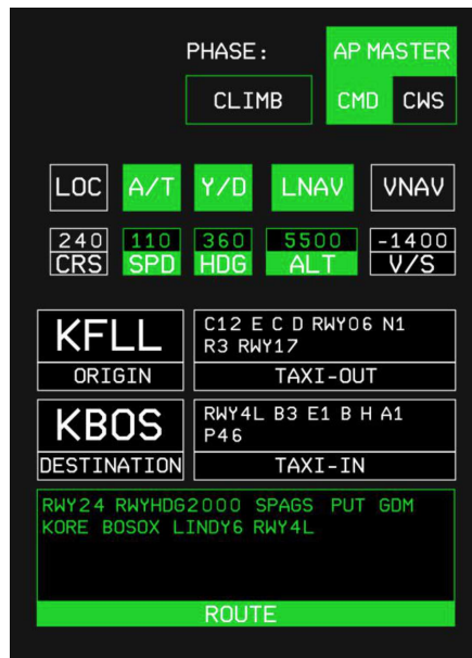
Figure F13: Autoflight Mode Control Panel
