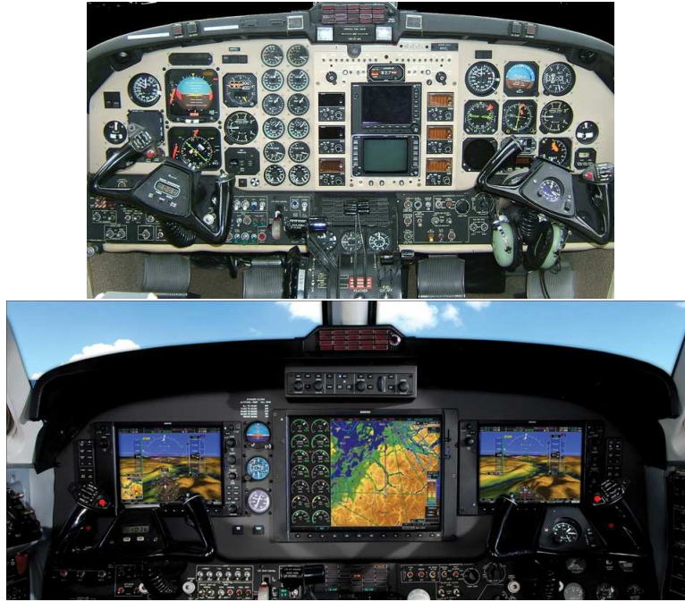
Figure F1: Comparison of Traditional vs. Glass Cockpits
