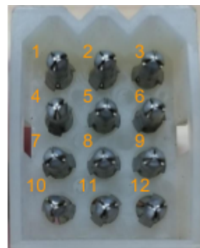
Figure B15: Audio Intercom Plug
