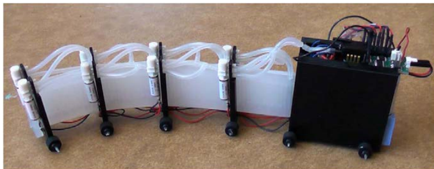
Figure 2 First experimental prototype of the soft robotics snake developed by Onal, Rus's group from MIT [6]
