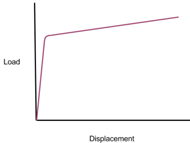
Figure 25: A basic load vs. displacement curve for the pneumatic application
