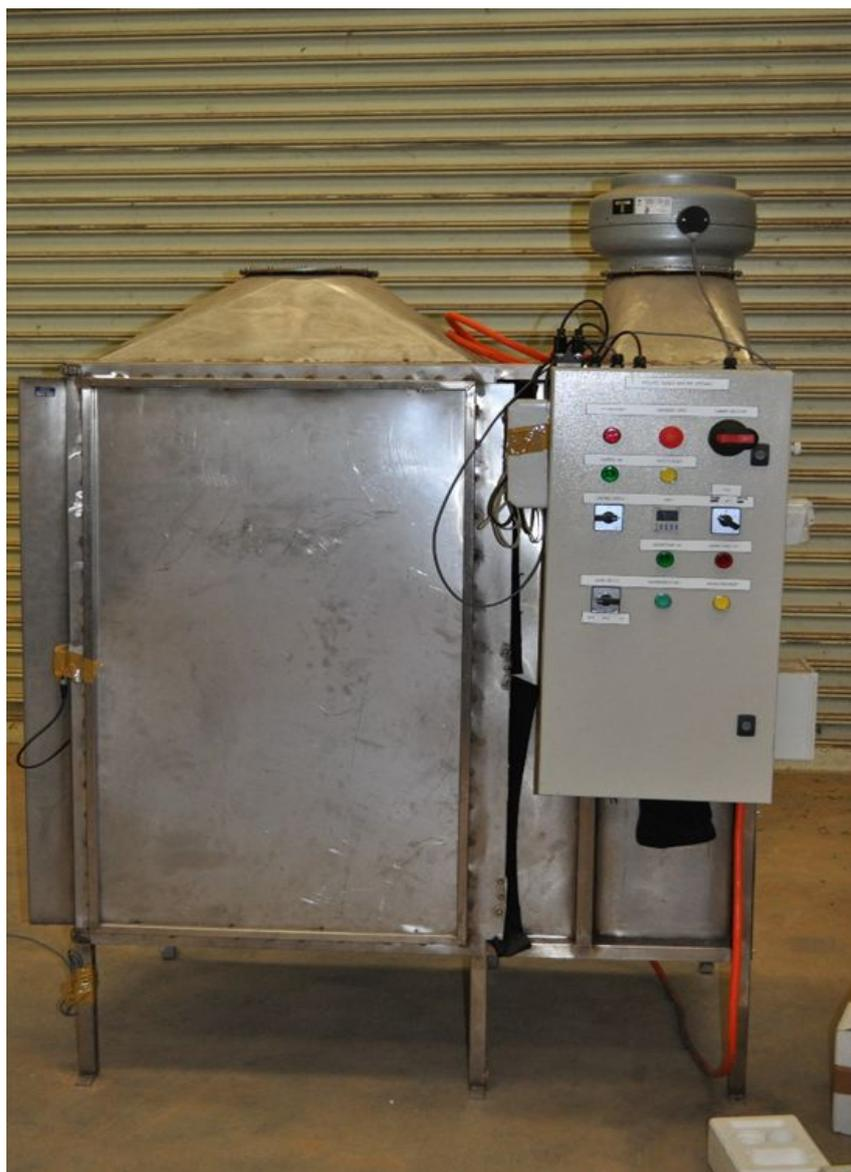
**Figure 13.** Microwave pyrolysis unit created and tested by Dr. Bhatta (2019).
